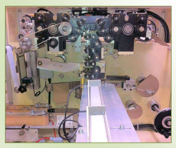
The SAS-PACKSAVON is our novel Soap Wrapper Family studied for simple applications. Its major feature is that it can wrap the soap bars with two films (inner carton stiffener and outer printed paper or BOPP). The wrapping style is double-point end fold.
